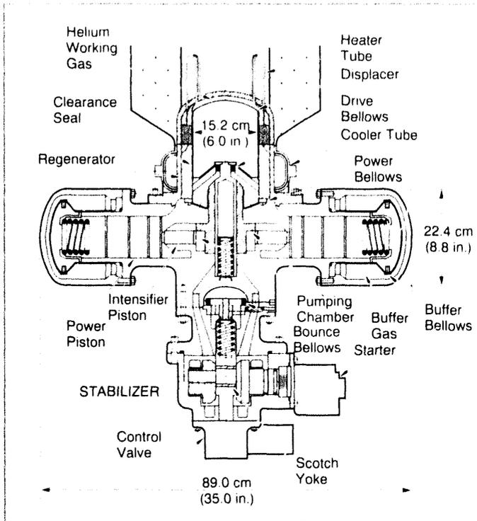
**Figure 4-4. The Stirling Technology Corporation STIRLIC™ 25-kW engine.**
