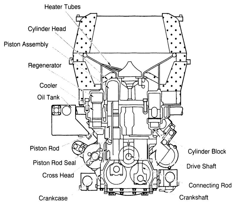
Figure 7-1. United Stirling 4-95 MKII Stirling engine.
