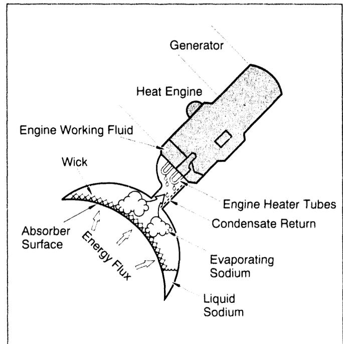
Figure 1-6. Reflux heat-pipe receiver.
