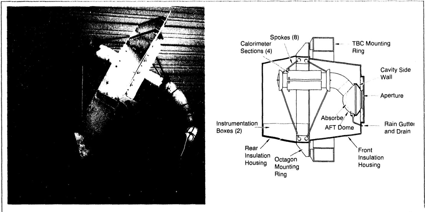
Figure 6-6. Sandia National Laboratories pool-boiler receiver.
