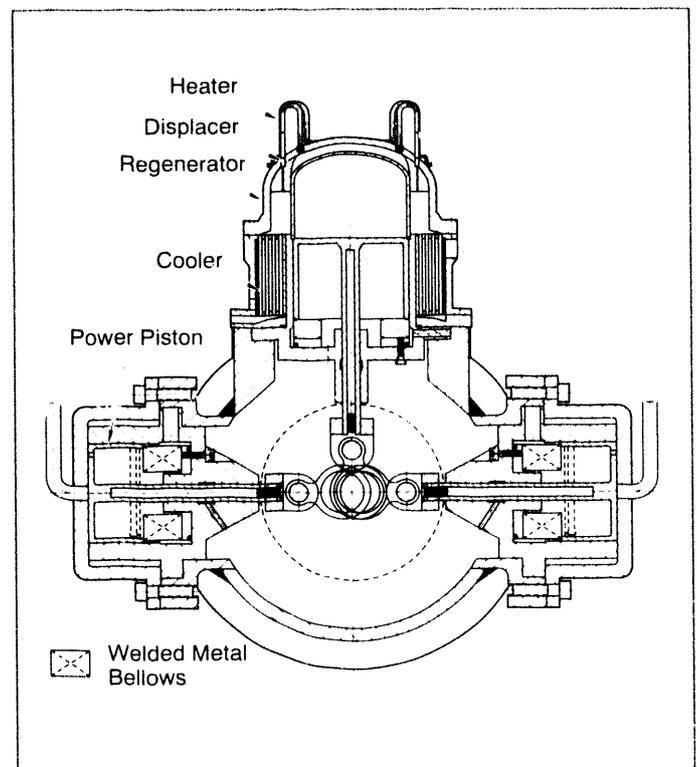
Figure 4-3. Stirling Technology Corporation 5-kW engine.
