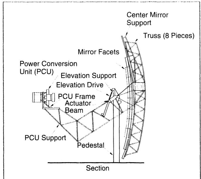
**Figure 1-2. Faceted parabolic dish concentrator with truss support.**
