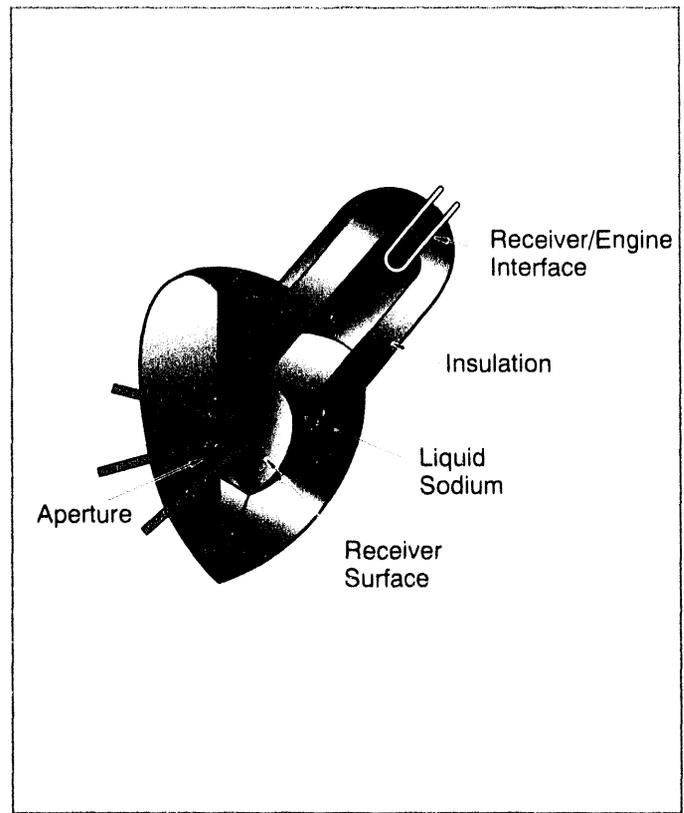
Figure 1-5. Reflux pool-boiler receiver.
