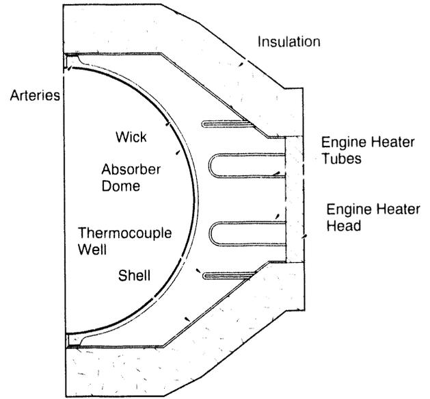
Figure 6-8. Cummins/Thermacore 35-kW<sub>t</sub> heat-pipe receiver.
