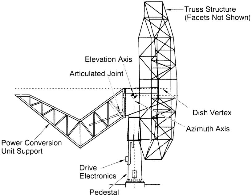
Figure 5-10. DOE faceted stretched-membrane dish development concentrator.
