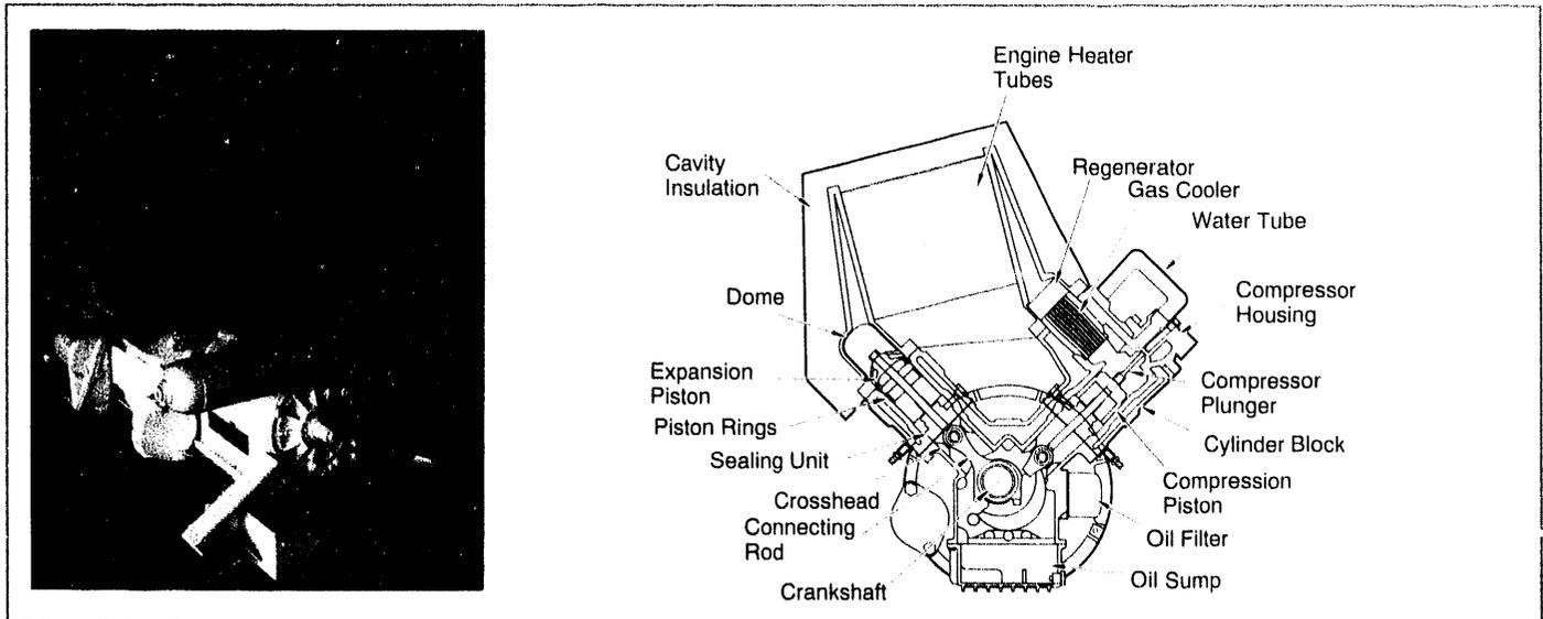
Figure 7-3. Stirling Power Systems/Solo V-160 Stirling engine.
