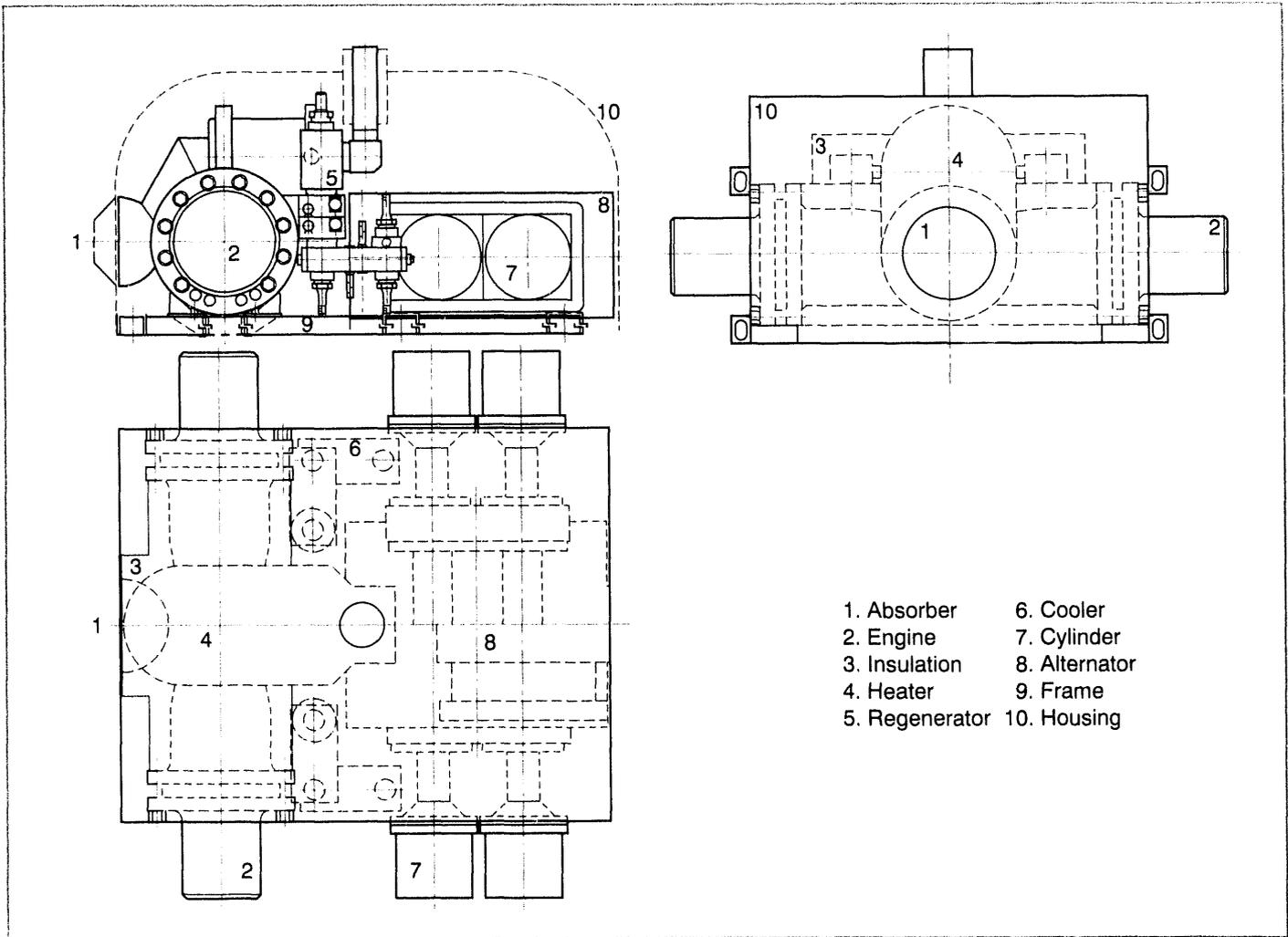
Figure 4-8. Russian free-piston Stirling engine.
