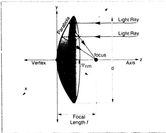
Figure 3-1. The paraboloid is a surface generated by rotating a parabola around the z-axis
