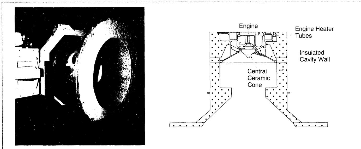
Figure 6-1b. United Stirling 4-95 engine with MDAC receiver.
