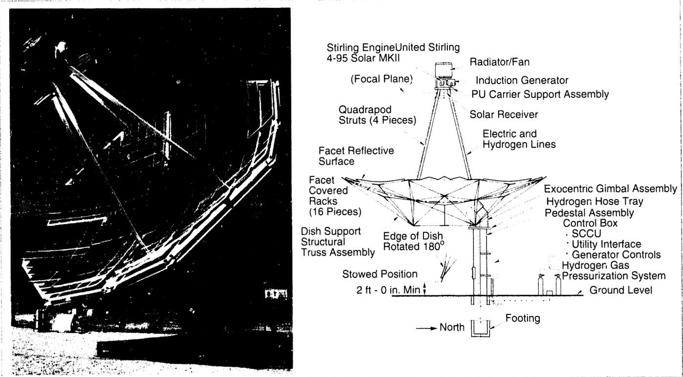
Figure 2-1. Advanco/Vanguard 25-kW<sub>e</sub> dish/Stirling system.
