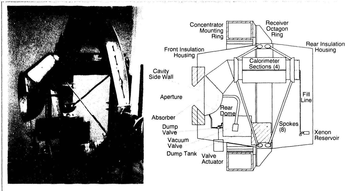
Figure 6-7. Sandia National Laboratories second-generation pool-boiler receiver.
