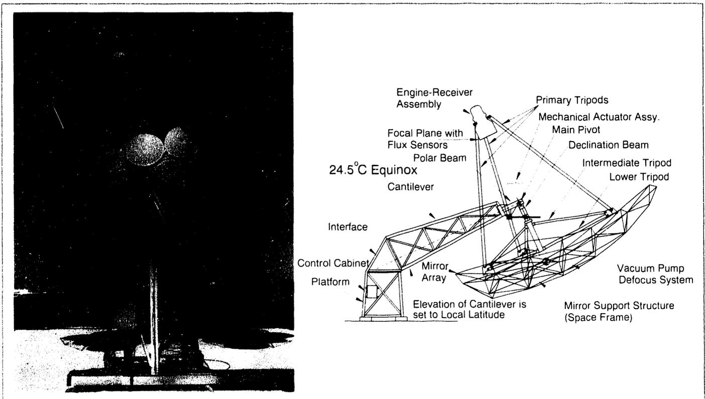
Figure 2-5. Cummins Power Generation 5-kW<sub>e</sub> prototype free-piston engine dish/Stirling system.
