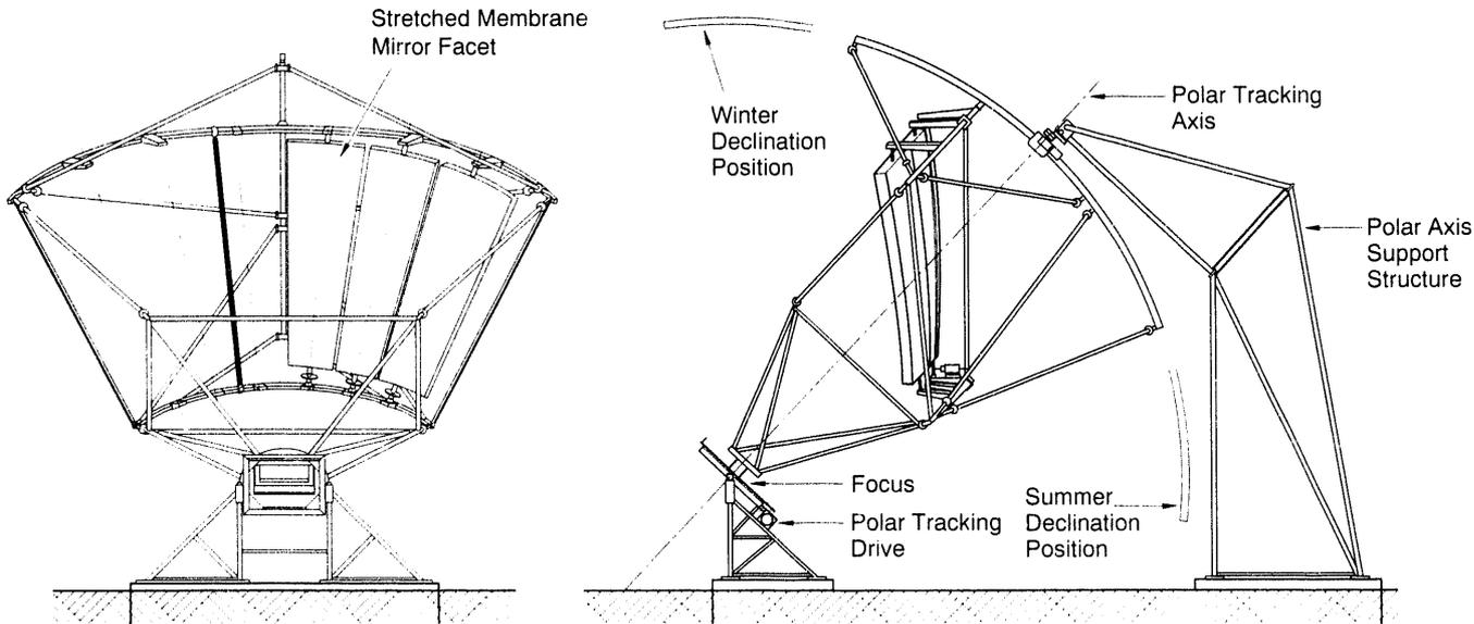
Figure 5-11. HTC Solar Research concentrator.
